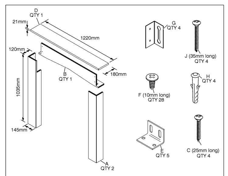
Figure 1. Contents (Items are not to scale. Any components extra to those above can be discarded).
